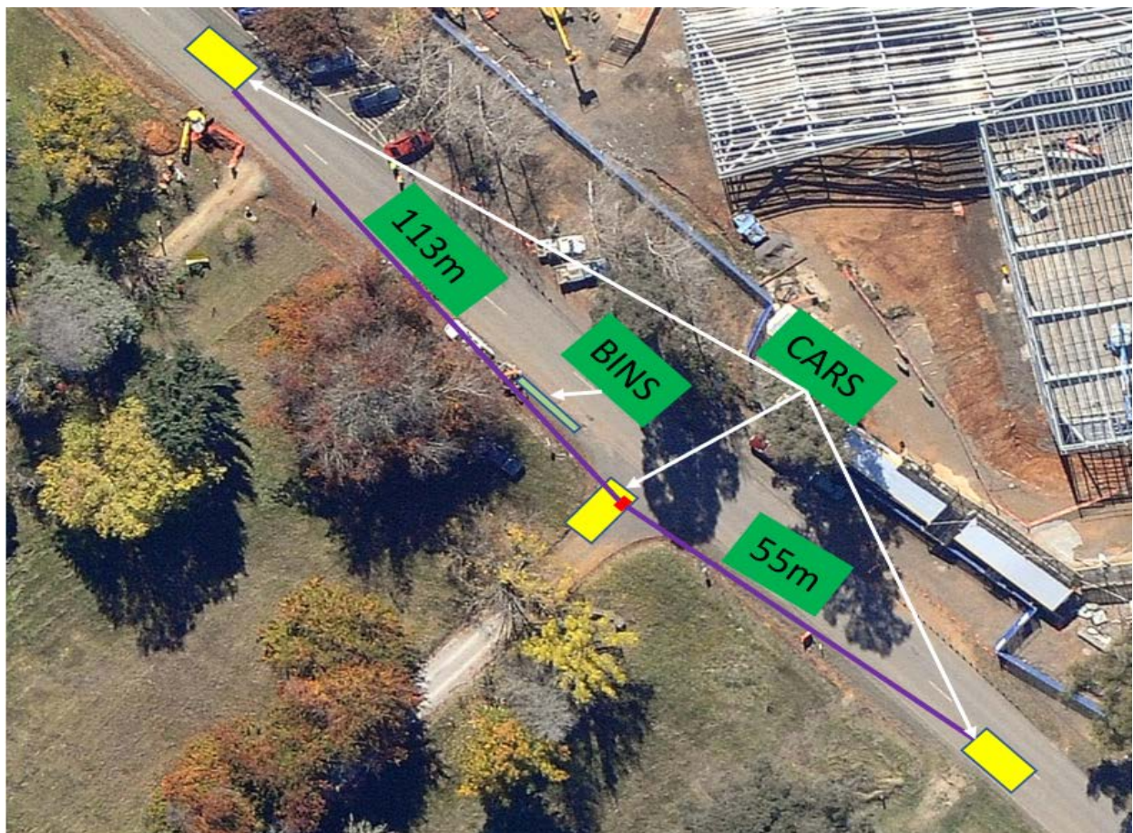
Figure 7 Sight distance assessment with the placement of the bins
