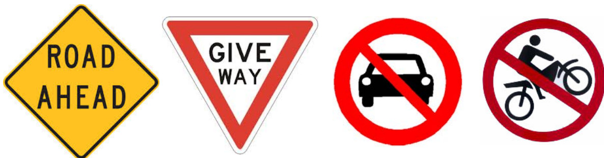
Above from left to right: Typical "Road Ahead" sign (W6-8); "Give Way" (R1-2); "No Motor Vehicles" and "No Trail Bikes" to be used on totem posts along the proposed rail trail.
