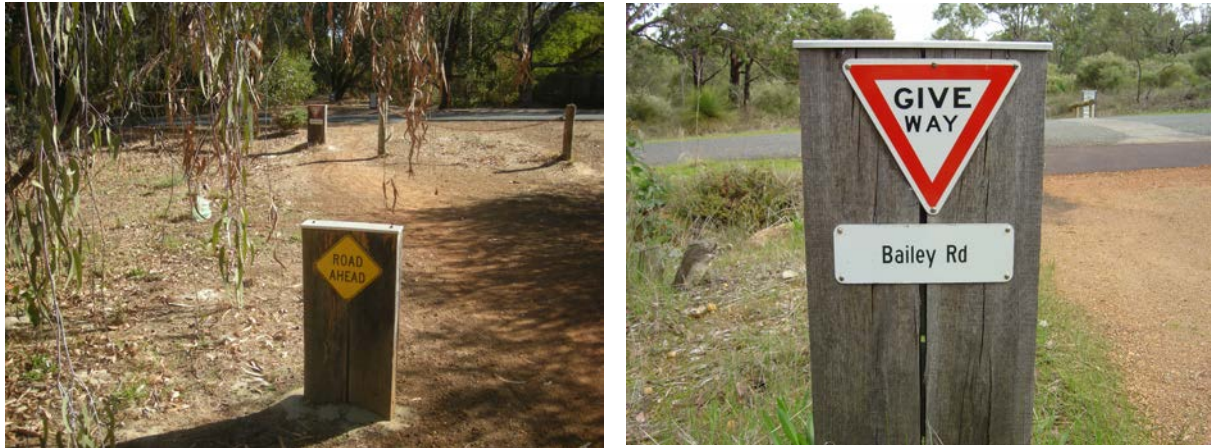
Above left and right: Road crossing signage is very important for trail users to alert them to the dangers ahead. On all major road crossings, a "Road Ahead" and a "Give Way" (or "Stop") sign are warranted. On minor road crossings, the use of a "Give Way" sign is considered sufficient. On-road "Trail Crossing" signs are also recommended at all road crossings.
