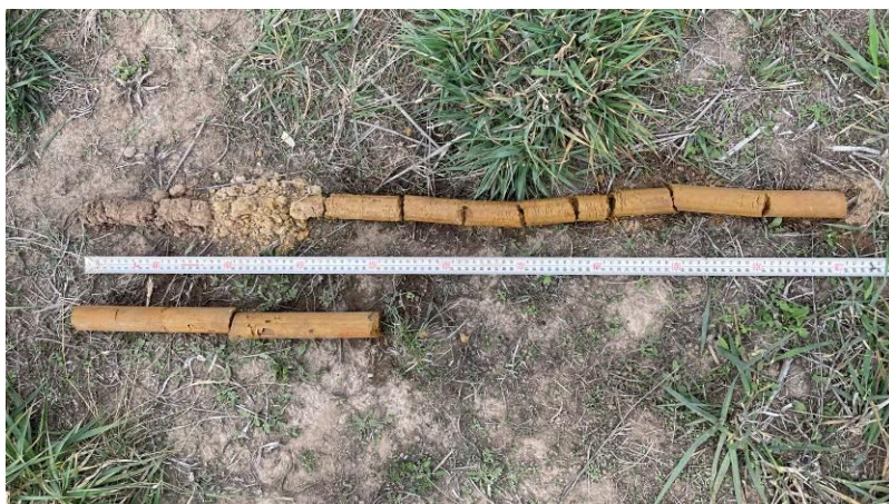
BOREHOLE BH 12 (Lot 12): Deep residual profile.
