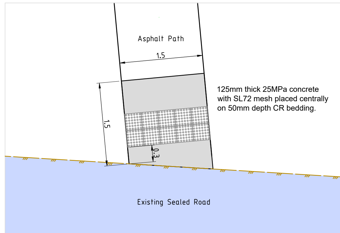
Typical Concrete Pad
