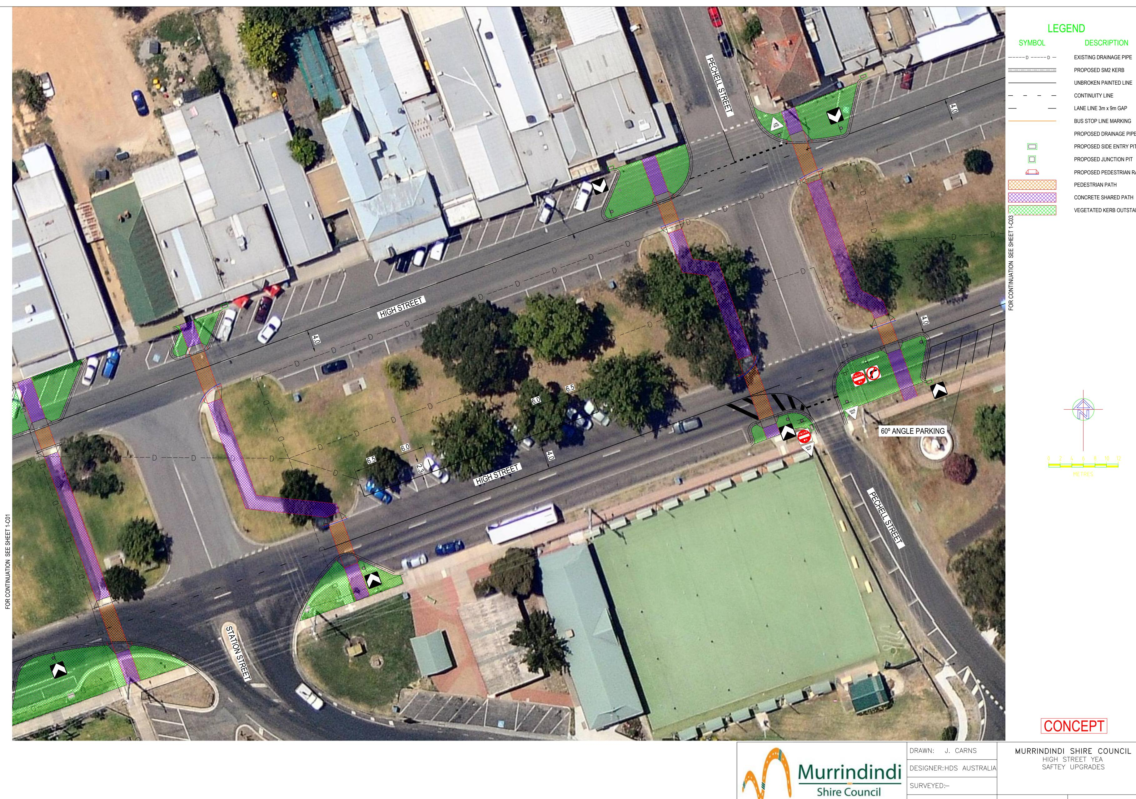
EXISTING DRAINAGE PIPE PROPOSED SM2 KERB UNBROKEN PAINTED LINE LANE LINE 3m x 9m GAP BUS STOP LINE MARKING PROPOSED DRAINAGE PIPE PROPOSED SIDE ENTRY PIT PROPOSED JUNCTION PIT PROPOSED PEDESTRIAN RAMP CONCRETE SHARED PATH VEGETATED KERB OUTSTAND
