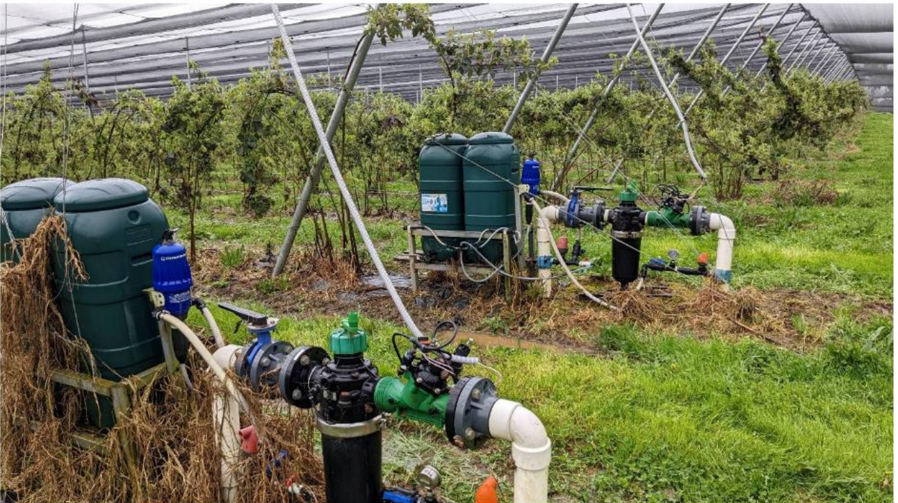
Image 4: Irrigation and fertigation equipment; every plant has a pressure-compensated dripper.
