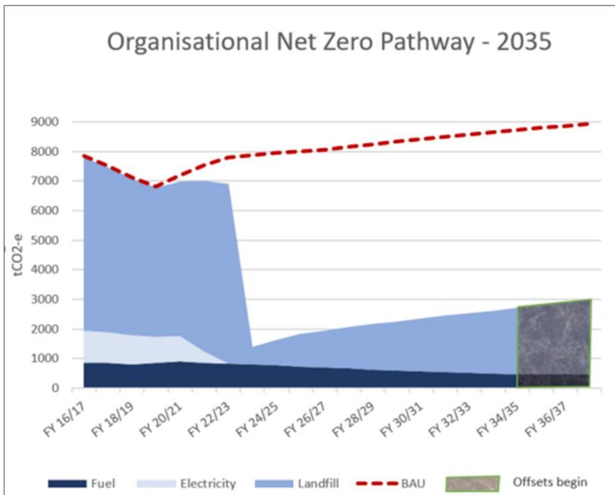
The sharp dip in the landfill profile in 2023/2024 is the result of capping the existing cells, which is programmed for around that time (the capping is presently being designed). The slight incline in the landfill emissions beyond that point is from progressively filling the new (western face) cells. This is despite combining food scraps with greenwaste (FOGO) in the kerbside collections after 1
