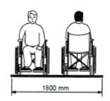
(d) To allow two wheelchairs to pass comfortably, a clear width of 1800 mm is required
